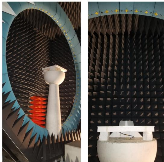
Figure 7: Test chamber pictures of the radiation pattern measurement setup
