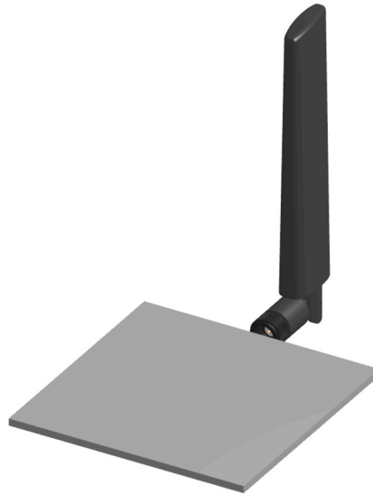
Figure 3. AC16000 Antenna at Edge of Ground Plane, Bent 90 Degrees
