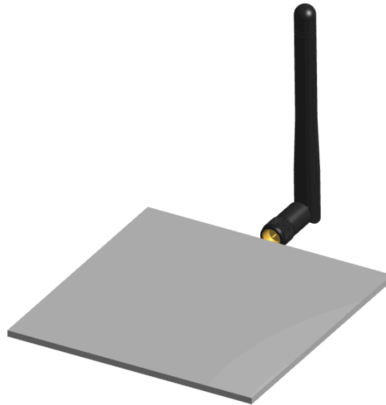
Figure 10. AC66503 Antenna at Edge of Ground Plane, Bent 90 Degrees
